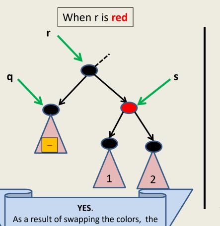
As a result of swapping the colors, the number of black nodes to the leaves of trees 1 and 2 unchanged. Interestingly, the deficiency of one black node on the path to the leaves of subtree(q) is also compensated. So we are done
