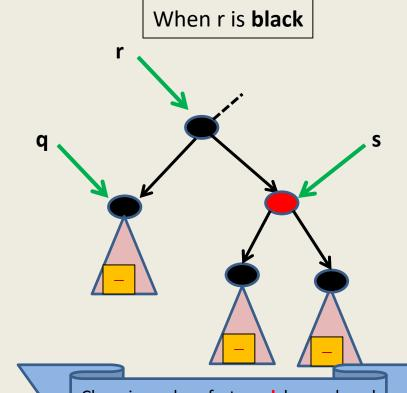
Changing color of **s** to **red** has reduced the number of black nodes on the path to the root of subtree(**s**) by one. As a result the imbalance of black height has *propagated* upward. So we process the new **q**.
